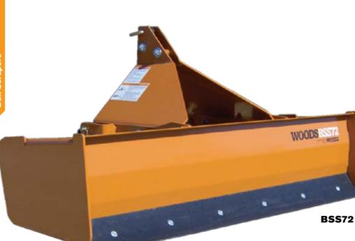
Tackle the toughest spreading and grading jobs with Woods<sup>®</sup> and Gannon<sup>®</sup> brand box scrapers. From the reinforced steel A-frame to the tough, reversible cutting edge and replaceable scarifiers, our box scrapers deliver exceptional durability and versatility.
