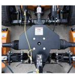
TRANSPORT LOCK QUICK RELEASE Easily pull the rope to release transport lock.
