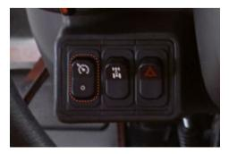
HST Cruise Control HST Cruise system enables the tractor to maintain a steady speed as set by the operator.
