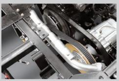
**Transmission** The MECHRON uses a continuously variable transmission(CVT) and has a time proven Daedong gear box with two speeds(Hi/Lo) and 4WD.
