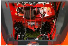
Spring Suspension Operator Platform Platform is suspended for comfort but can also be stowed away allowing the operator to walkbehind the mower for tight or confined areas.
