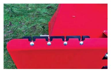
Replaceable, serrated tow bar strip
