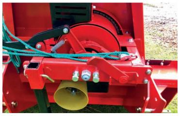
**Replaceable cable drum frame** All forest winches in the V-series are now delivered with an easily removable cable drum frame, which facilitates servicing or replacement of drive *chain* or clutch parts.
