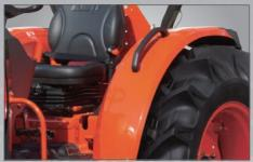
**Fender Grip** Available on each side of ROPS model tractors, these handles provide assistance while getting on and off of the tractor.
