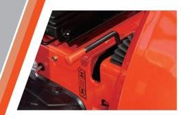
**4WD Engagement** The 4WD comes standard on all models and is engaged with an easy access lever.
